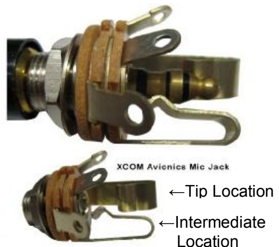
Microphone jack has two terminals and earth
