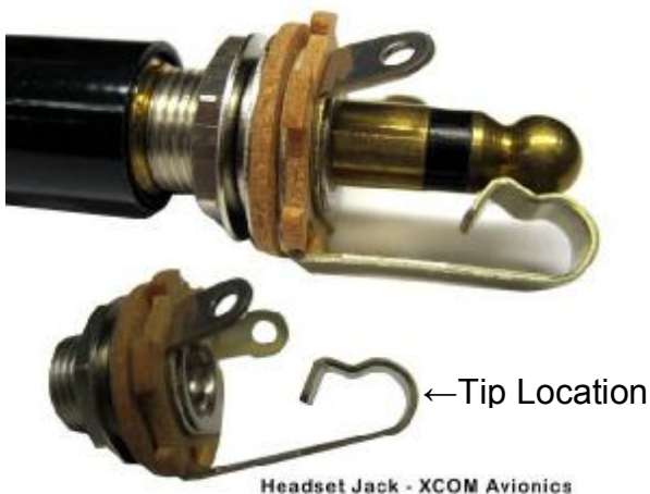
Headset jack has one terminal and earth
